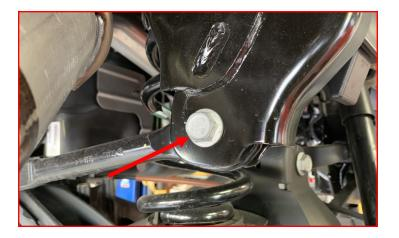
Remove parking brake bracket mounting bolts from the lower control arm on the driver side. Retain the hardware.
