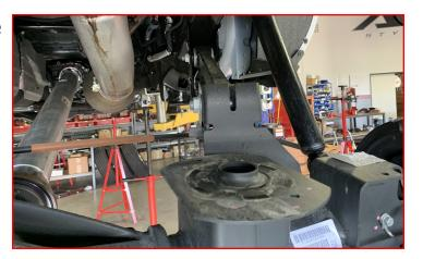
Install the coil spring with coil spring spacer and isolator. Raise the axle high enough to keep springs and spacers in place.
