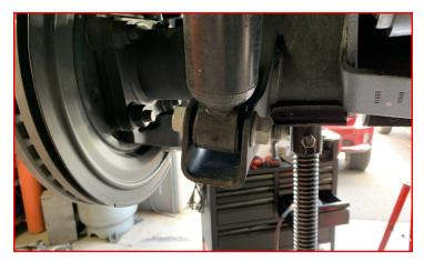
Loosen the track bar at the axle and frame mounts but do not remove.
