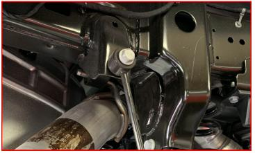
Install the parking brake bracket the lower control arm on the driver side using the factory hardware.
