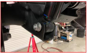
Install the sway bar end links to the frame using the factory hardware.
